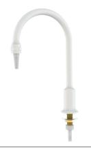
Application: Deck mounted polypropylene-lined gooseneck for distilled, deionized and reverse osmosis water. Fitting has exterior brass casing and interior lining of inert polypropylene. Pure water comes in contact only with inert plastic.
